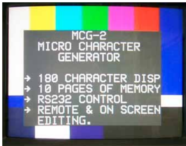
Raster output of MCG-2 over SMPTE bars
